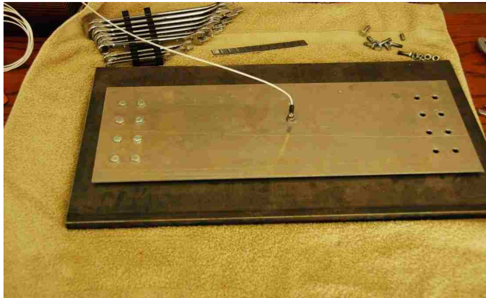
Figure 2.5: Photo of Aluminum Test Plate Setup
