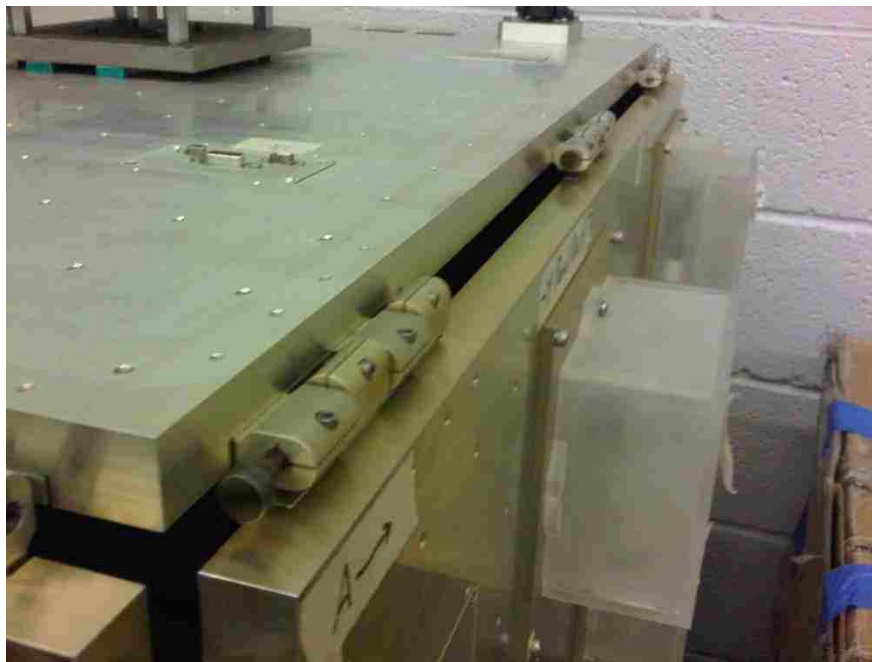
Figure 4.9: Photo Showing Connection Between Panels on Mock Satellite
